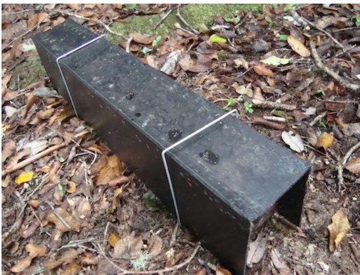
*These are short tunnels which can be made from a simple corrugated plastic such as the Coreflute® or Correx® material used in chewboards. Onto the floor of the tunnel is placed a special tracking card (500 x 100mm) that records the footprints of animals that enter the tunnel.*
