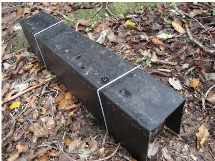
*These are short tunnels which can be made from a simple corrugated plastic such as the Coreflute<sup>®</sup> or Correx<sup>®</sup> material used in chewboards. Onto the floor of the tunnel is placed a special tracking card (500 x 100mm) that records the footprints of animals that enter the tunnel.*
